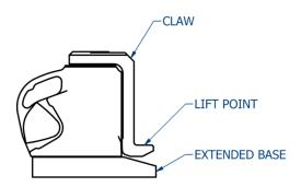
The capacity of the claw is 40% of the capacity of the jack to which it is fitted (See table 1), if the claw is overloaded it could snap and put the operator in danger. Jacks intended for use with claws have extended bases which prevent the jack from toppling over when a load is applied to the claw. Never attempt to use a claw on a jack without an extended base. They must only be used for vertical movements of loads.
