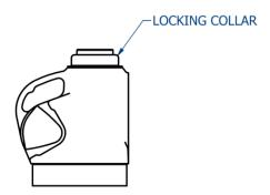
All models can be provided with screwed rams and locking collars. The purpose for this is to mechanically support a load at a required position without relying on the hydraulic circuit.
