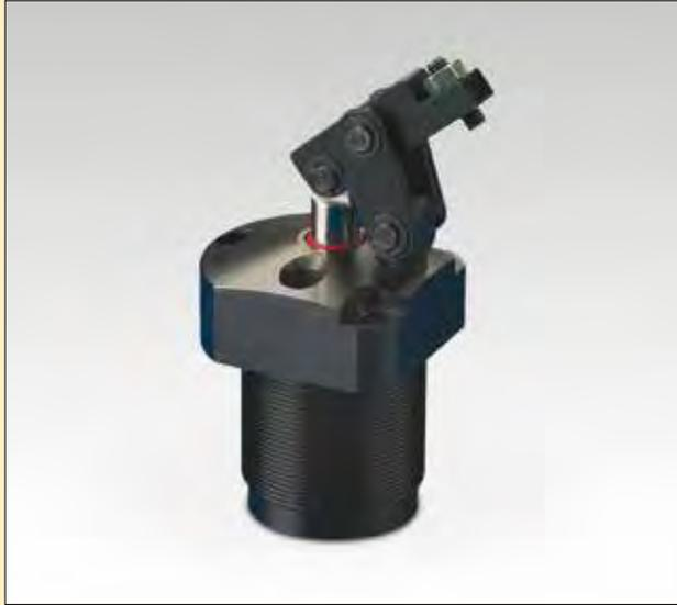
**Link clamp allows unobstructed part loading and high clamping forces. The hydraulic cylinders extend to provide clamping force, and retract to allow part removal.**
