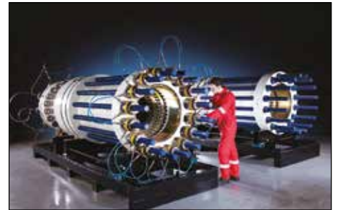
▲ Inter-connected with HT-Series hoses Enerpac subsea tensioners apply uniform bolt load.
